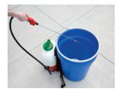
Repeat the procedure with clean water until the tank is thoroughly clean. Wash outside of nozzles and dry with a cloth.
