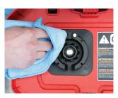
Keep electrical contact posts between bottom of tank and base clean.
